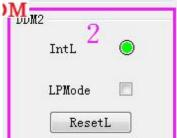
IntL -- module malfunction warning light: red means malfunction, green means normal working; LPMode -- low consumption mode: close each channel light of the module; ResetL -- module restoration: DDM value reset.
