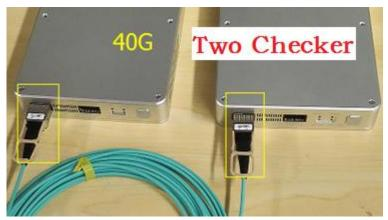
Note: One end module of AOC&DAC connected to one port of one checker, another end module connected to one port of another checker.
