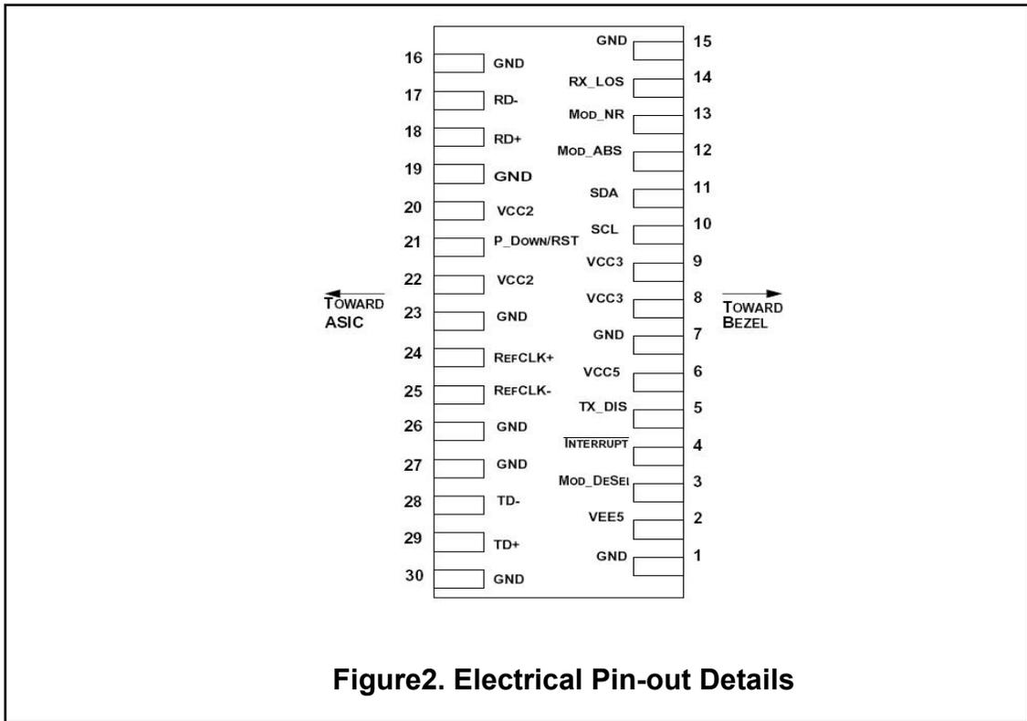
Figure2. Electrical Pin-out Details
