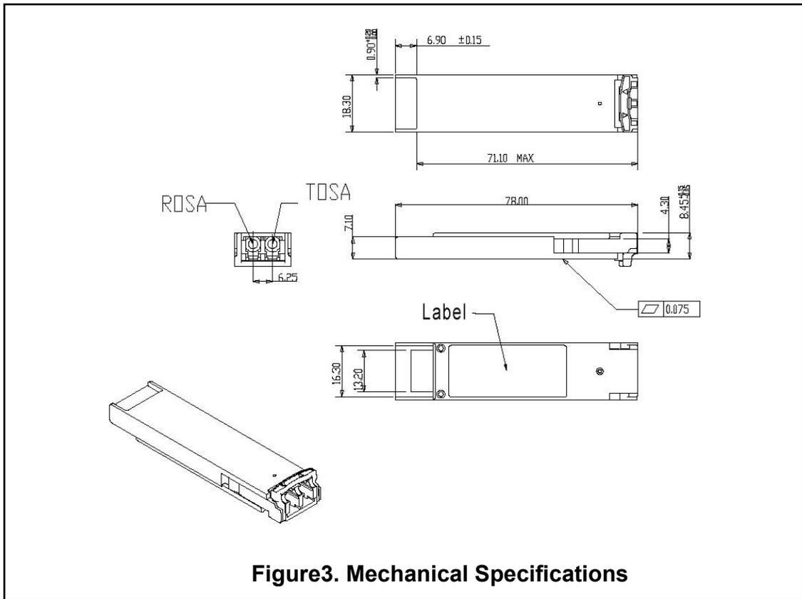
Figure3. Mechanical Specifications
