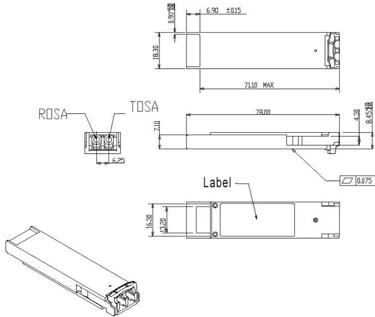
**Figure3. Mechanical Specifications**
