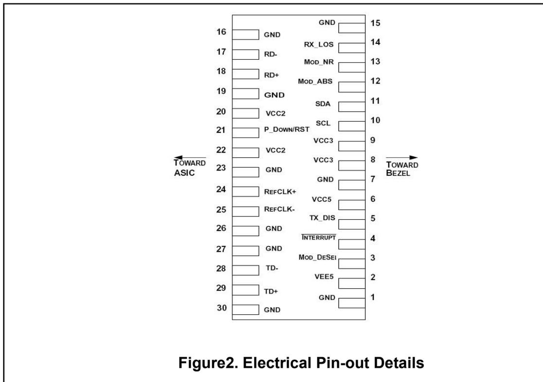
**Figure2. Electrical Pin-out Details**
