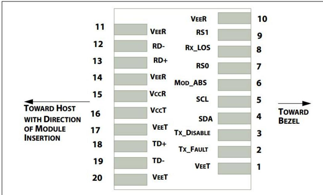
Figure2. Host PCB SFP+ pad assignment top view
