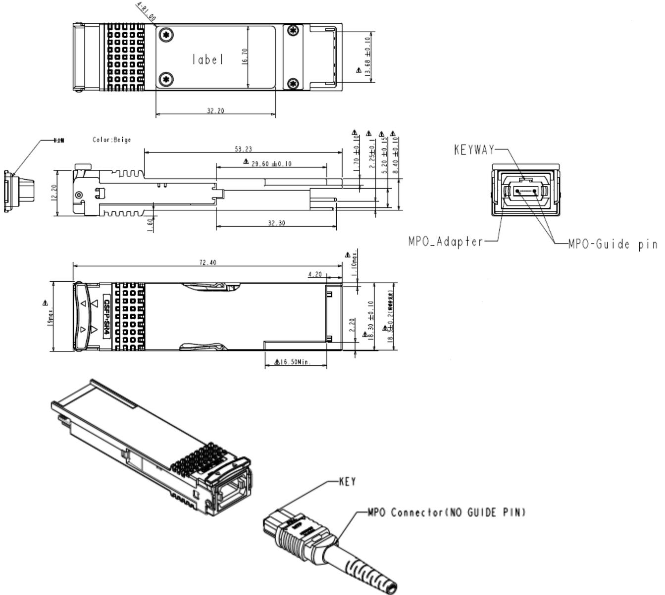
**Figure10. Mechanical Specifications**
