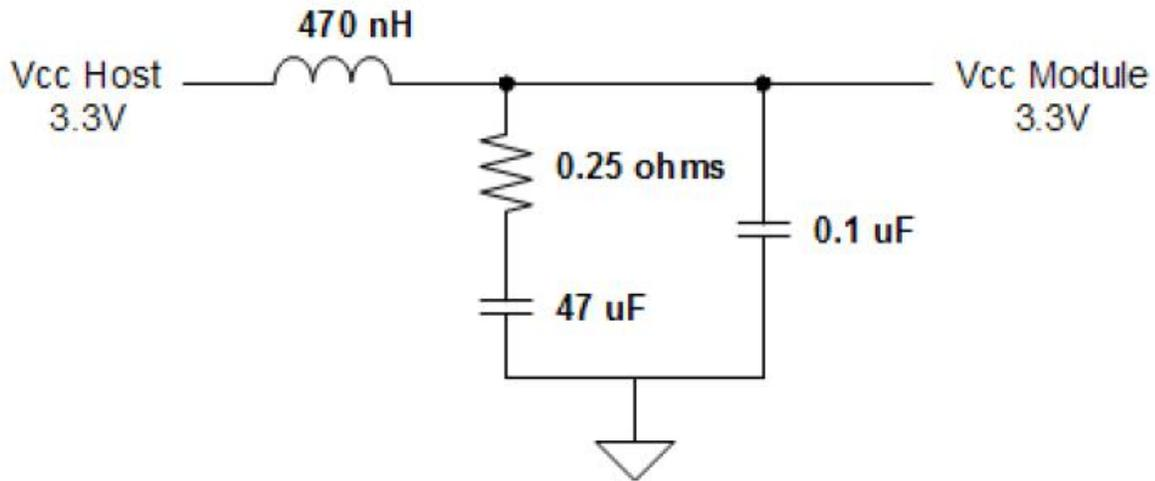
The host board should use the power supply filtering shown in Figure3.
