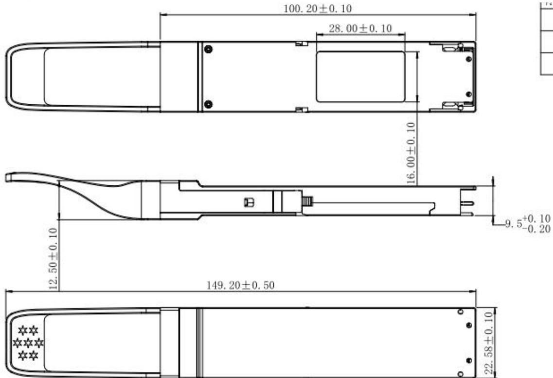
**Figure6. Mechanical Specifications**
