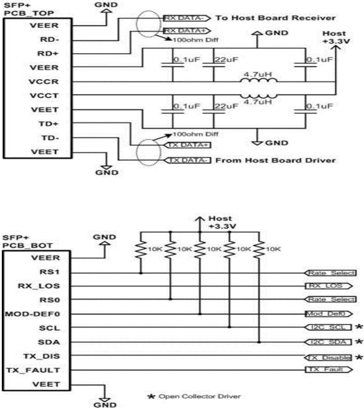
Figure 3. Recommended Interface Circuit
