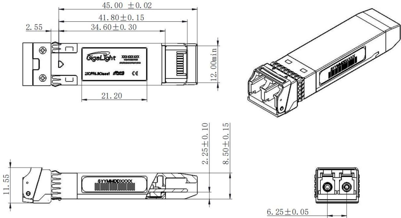
**Figure 5. Mechanical Specifications**
