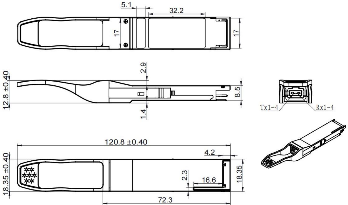
Figure 12. Mechanical Specifications
