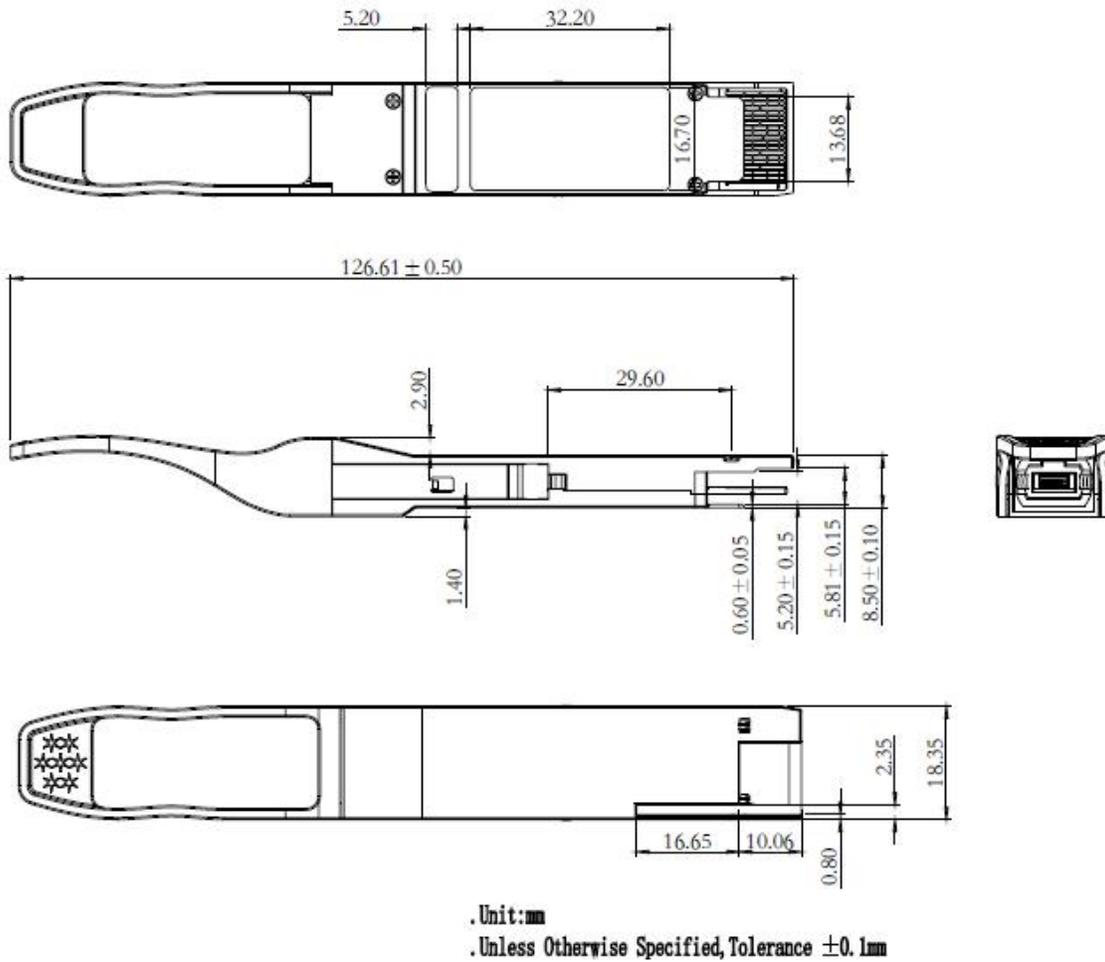
Figure10. Mechanical Specifications
