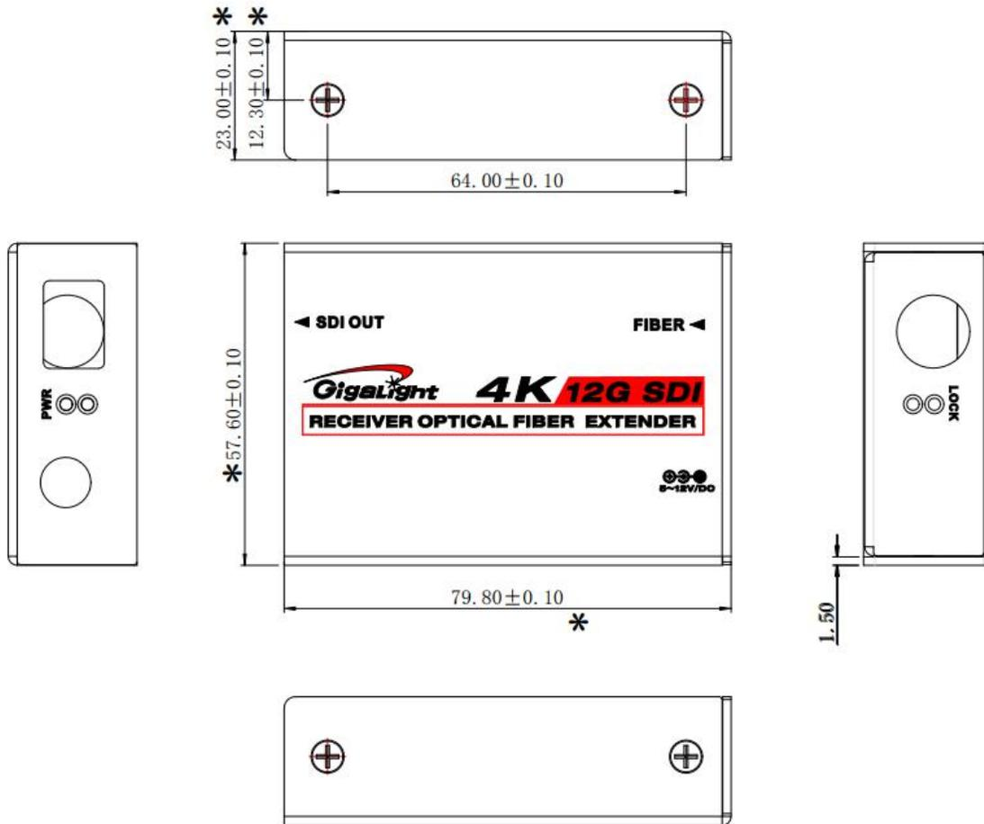
Figure 2. Mechanical Specifications
