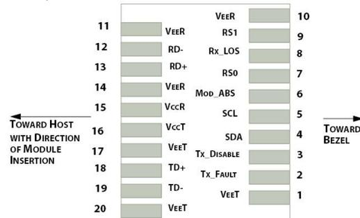
Figure2.Electrical Pin-out Details
