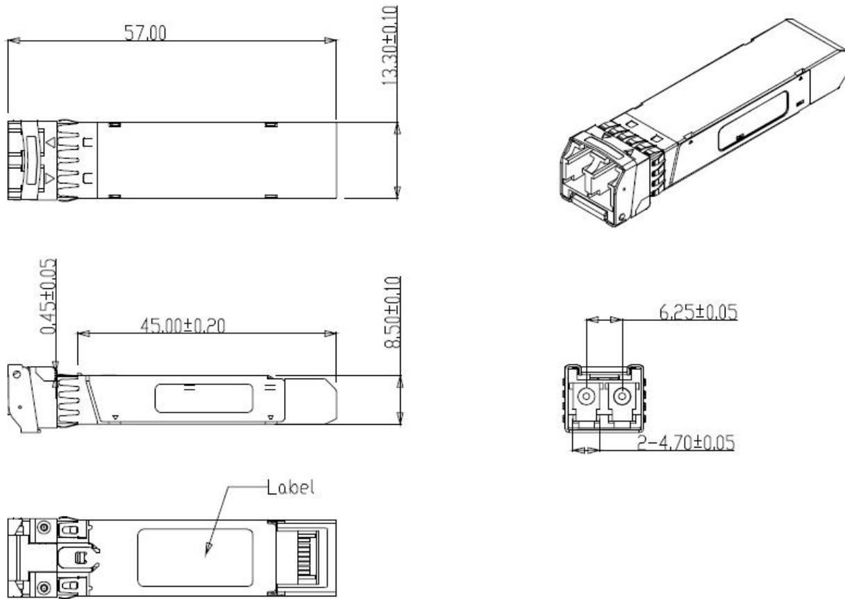
**Figure5. Mechanical Specifications**
