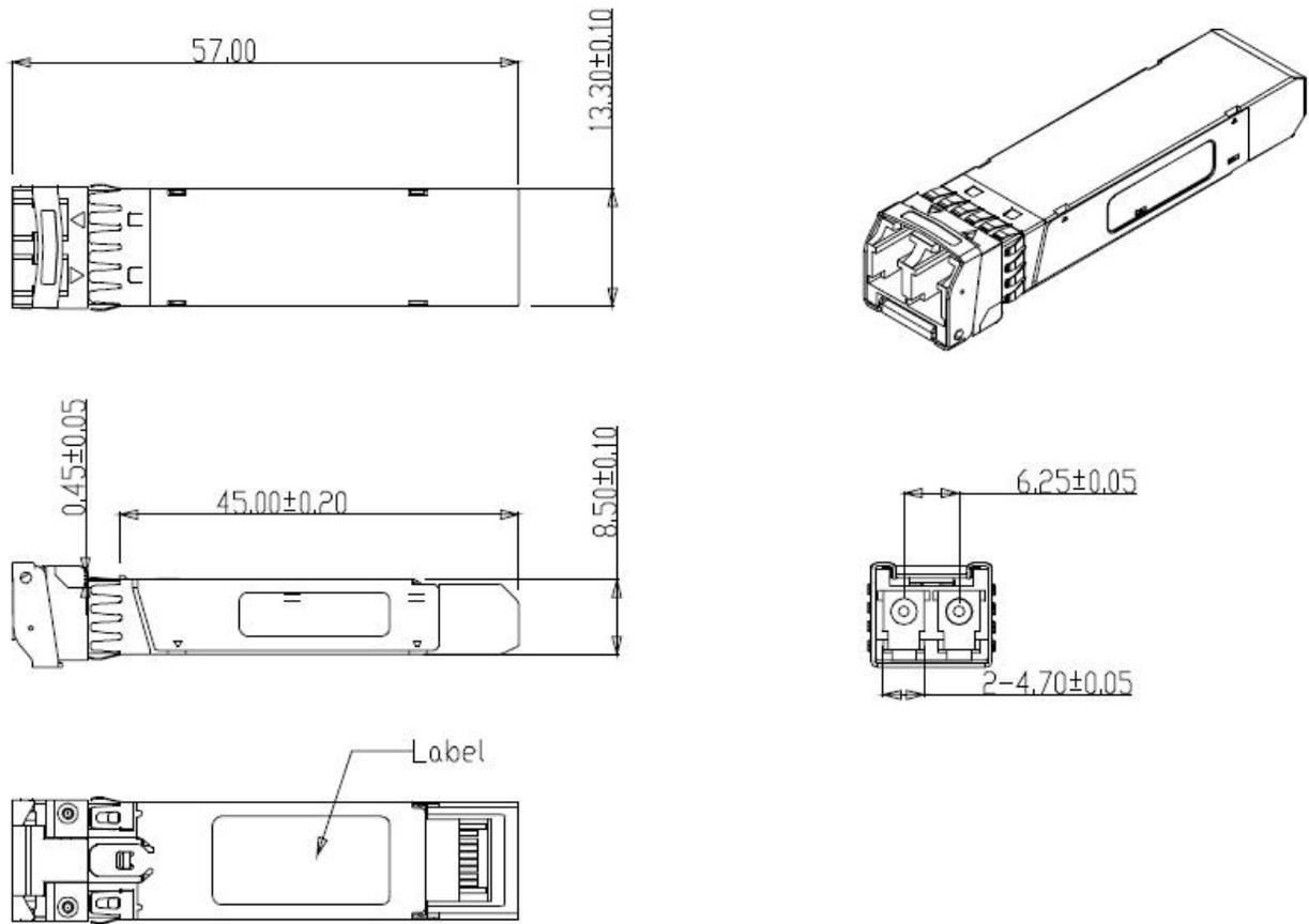
**Figure5. Mechanical Specifications**
