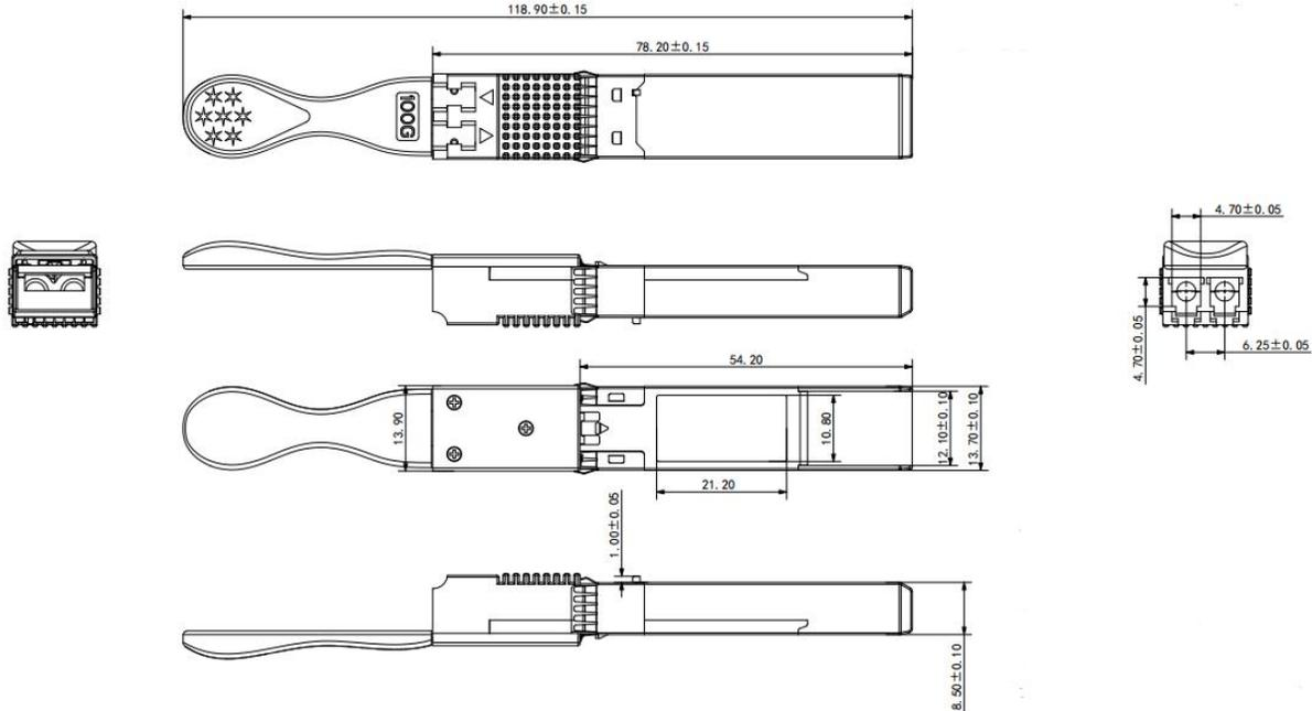
**Figure 8. Mechanical Specifications**
