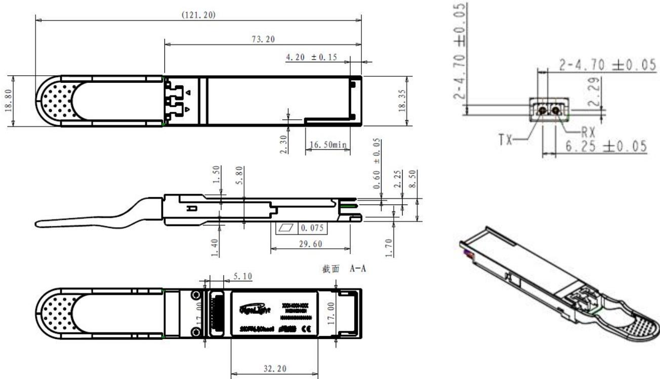
**Figure10. Mechanical Specifications**
